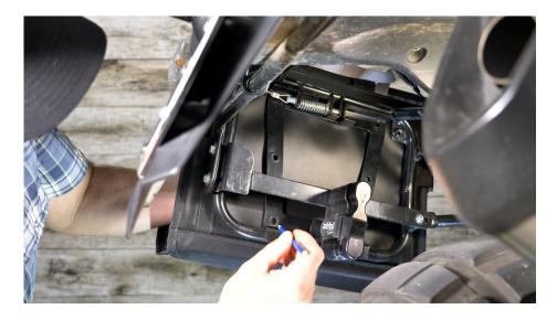
Do not mark any upper attachments at this stage. If you have upper attachments, you will want to mount your lower attachments first as this will allow you to set the Holster back into the frame rack while you mark for the upper attachments.
