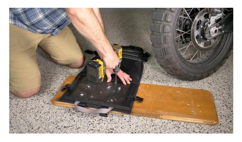
We recommend using a scrap piece of wood under the Holster while drilling to prevent damage to your drill or floor.
