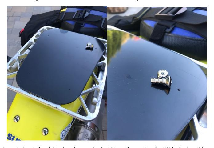
Determine length of needed hardware by measuring the thickness of your rack, adding 1/8" for the plate thickness, and then a min of ¼" for the locking nut. We do recommended to use a button head or pan head type screw. Using a countersunk type screw (pictured above) will require use of an appropriate supporting washer. Always use a locking nut to prevent loosening of hardware.
