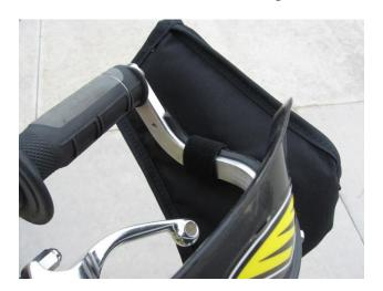
2) Now fold/re-invert the Grip Mitt inward and over the hand guard and grip. Select which button snap position allows for the best angle of the Velcro strap. Overlap the lower and upper Velcro strap to secure the Grip Mitt around the handlebar.
