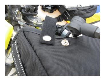
Make sure that the Grip Mitt and/or Velcro straps do not interfere with any of the motorcycle hand controls.
