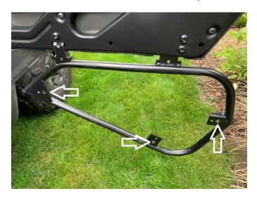
2) With the outer panel now removed from the lower door frame find the correct side bag. (Lower Door Bags are left/right specific) Start by attaching the one wrap
