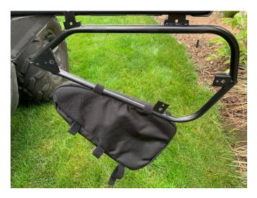
3) With the Lower Door Bag in place now attach the upper one wrap hook and loop to the upper rail of the door frame. Remember, it is best to fully wrap the frame rail with the hook and loop. (The hook and loop tabs on the bag have been intentionally left a bit long. Trim back as needed with sharp scissors)
